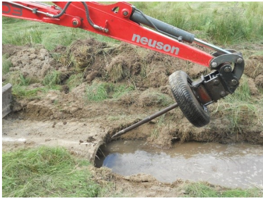
Bespoke pipe extraction attachment on digger, in operation.
